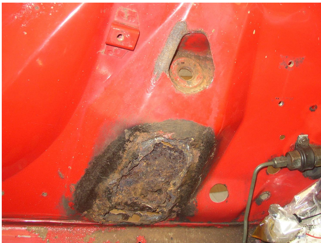
Inner wing corrosion
