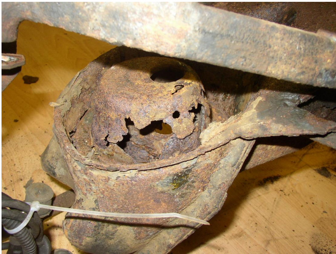
Sub-frame spring turret cone
