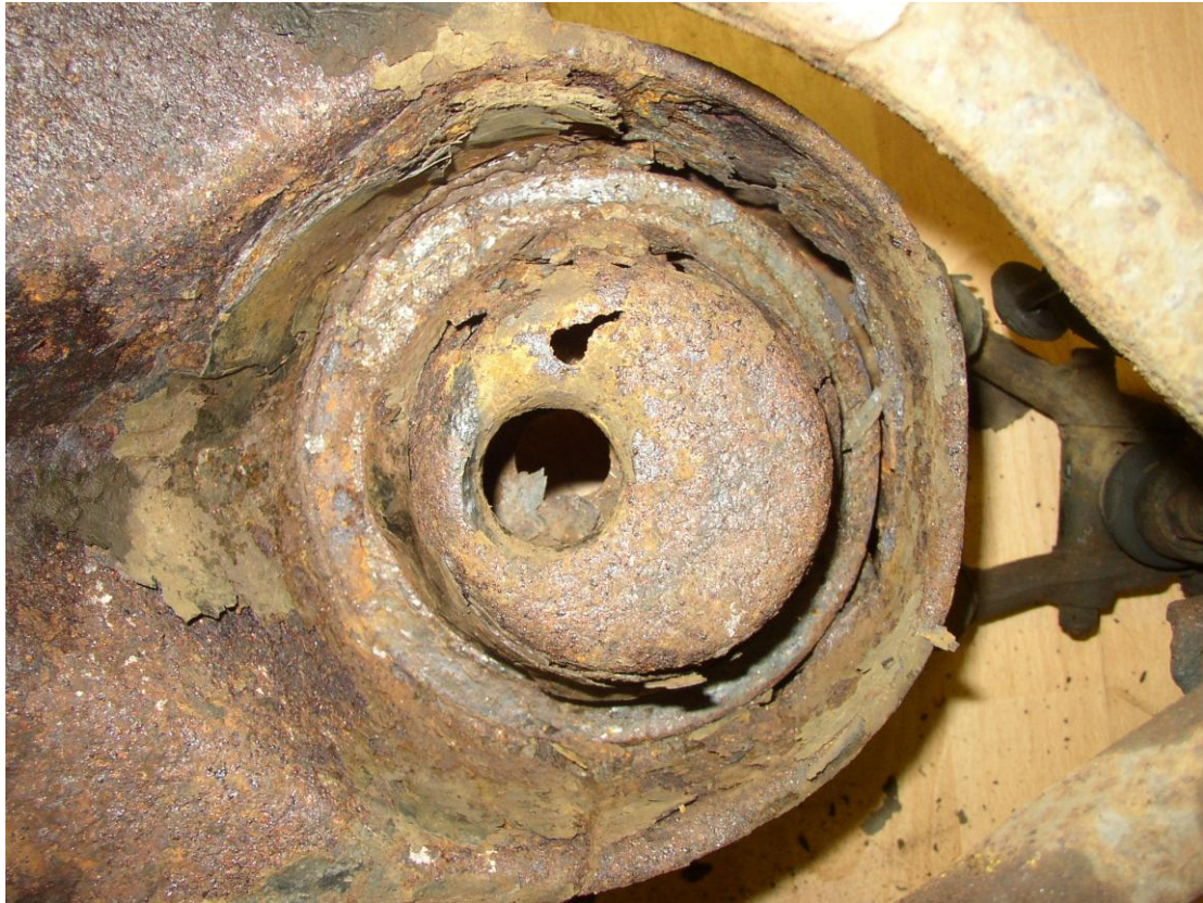
Sub-frame spring turret showing spring base
