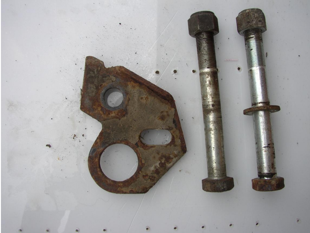
Front sub-frame mounting bolts and tow bracket
